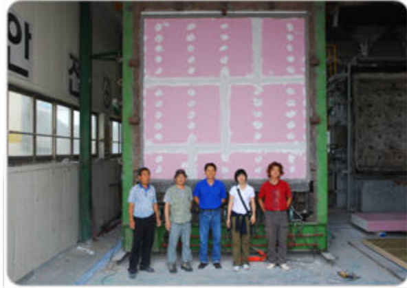
Canada Wood Korea Fire Tests Conducted at KICT: Two 2x4 wood framed walls, one for interior and the other for exterior wall, were built with No. 2 grade, Canadian S-P-F lumber by attaching two layers of 12.5 mm thick fire rated gypsum wallboards
