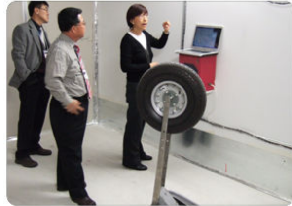
The "Tire Drop Test" for Impact Sound
